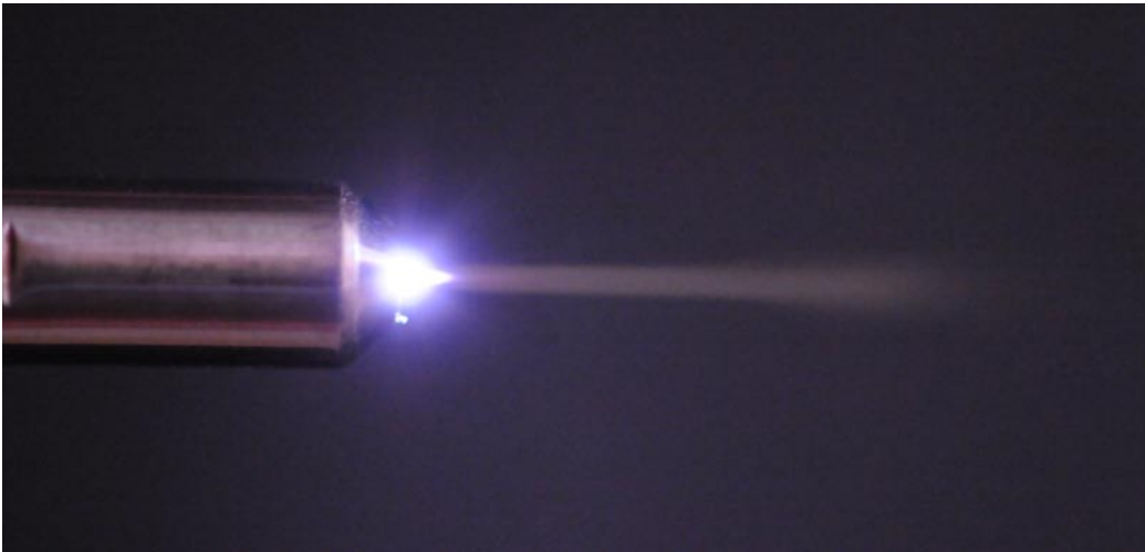
Fig 3 Plasma stream emerging from the tip of the PlasmaJet® handpiece
